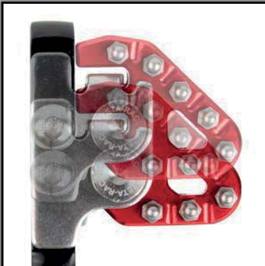
Designed to prevent sand and mud from entering tip folding area from front and side of brake tips.
