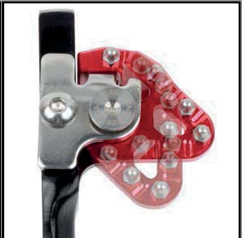
Thin tip design to prevent it from hitting the ground. Designed to prevent sand and mud from entering the tip folding area from front and side of brake tips. Pins are designed for sensitive pedal control and traction.
