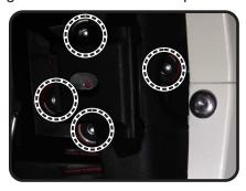
4. Remove the four fender mounting collars from subframe as they will not be used with the Yoshimura fender eliminator kit.
