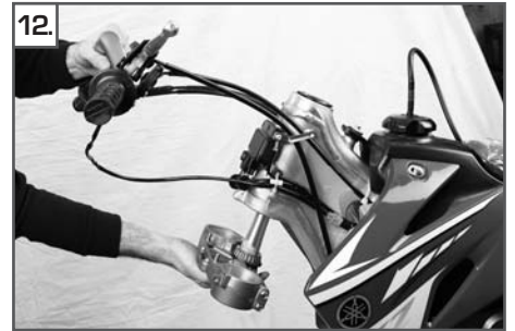
12. Remove the lower triple clamp. Clean the motorcycle's steering head and bearing seat.
