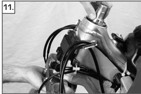
11. Holding on to the lower triple clamp, remove the adjusting nut on the steering head bearing.
