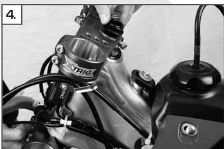
4. Mount the upper triple clamp and screw the adjusting nut ( 4 ) on by hand.
