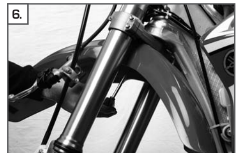
Remove the fender.
