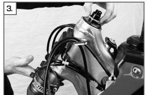
3. Depending on the model, mount the seal for the steering head bearing (sealing washer or O-ring)
