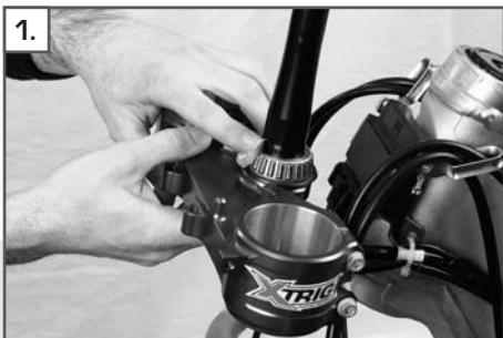
1. Grease the steering head bearing on the pre-assembled XTRIG triple clamp with suitable bearing grease.
