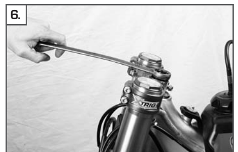
6. Use the adjusting nut ( 4 ) to adjust the desired bearing clearance.
