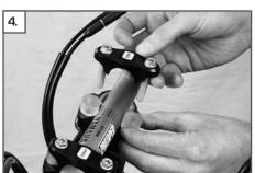
Mount the upper pan (7) with the preassembled intermediate rubber (8), screws (10) and elastomers (9).
