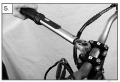
Evenly turn in the screws ( 10 ) and tighten to 16 Nm, making sure the clamping gap between the pans ( 6 ) + ( 7 ) is the same size (see photo correct/incorrect).
