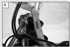
Mount the handlebar and move it into the desired position.
