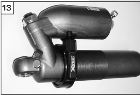
Make sure not to screw the Preload Adjuster all the way to the end of the thread since this can damage the thread.
