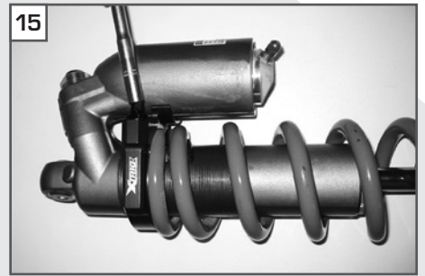
Preload the spring through the Xtrig Preload Adjuster and make sure the spring retainer is in the correct position.
