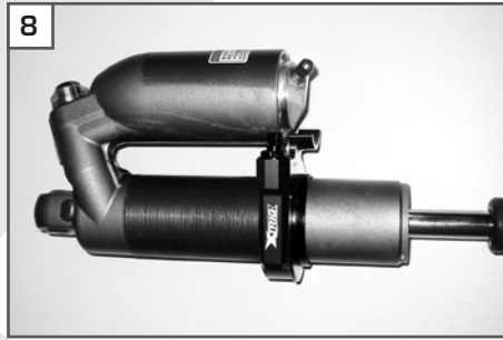
Slip the Xtrig Preload Adjuster on the shock absorber.
