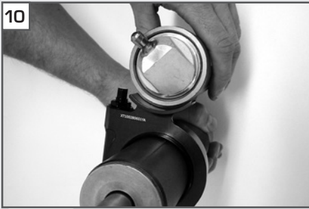
Make sure the Preload Adjuster mount is in the correct position to keep it from blocking, which can damage the thread.
