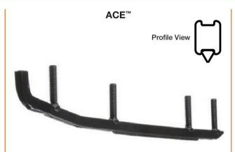
The ACE™ runner line utilizes a preformed steel square bar. It has a taller profile and is more aggressive, providing excellent control on rider forward sleds. The ACE™ is great for deep snow and is available with 6" and 8" of 60° turning carbide for trail users in our most popular runner lines.
