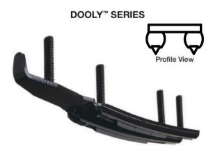
The Dooly<sup>™</sup> runner will help decrease darting of your sled as it makes its own groove in the trail. The tucked front end will ensure stability. The two 7/16" Flat-Top® runners mounted on a plate are available in 4", 6", or 8" of 60° turning carbide to accommodate several styles of trail riders. Each Dooly<sup>™</sup> runner is packaged individually.
