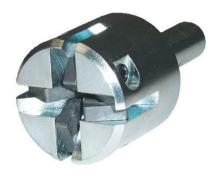
Our stud sharpening tool is easy to use and will sharpen your studs while they remain in the track. Available in 30° (TOOL-SHARP-3), 45° (TOOL-SHARP-4), and 60° (TOOL-SHARP-6) angles. Replacement inserts are available in packages of 4 (TOOL-INSERT-4). Use with steel studs only.
