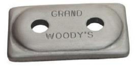
Double Grand Digger® support plates are specifically designed for use with the 5/16" Grand Master® stud lines in a single-ply track. This lightweight support plate allows you to install two studs with less weight than two single support plates. This aluminum support plate also increases your options for studding in the middle belt.
