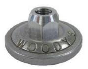
Available for two-ply tracks, the Combo Digger® support plate is the perfect combination. The nut and support plate are affixed together, making it unique, easy to install, and a time saver. This aluminum support plate is only for 5/16" studs that are 1.325" and longer. Available in quantities of 24 and 48.
