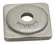
Grand Digger® support plates are specifically designed for use with the 5/16" Grand Master® stud lines in a single-ply track. Square aluminum support plates must be indexed to perpendicular with the edge of the track. The indexing tool, SPI-TOOL-G, to align Square Grand Digger® support plates is available from Woody's® (page 16).
