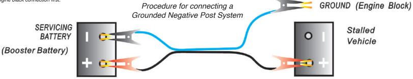
\* For positive ground vehicles (predominantly found only in pre-1956 vehicles) ground the negative clamp, and leave the positive clamp connected to the positive terminal on the stalled vehicle battery.
