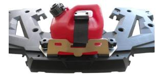
• Before each ride make sure the bracket is firmly fixed to the rear rack and the buckle straps are securely fastened to the gas can.
