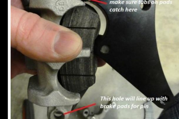
Mount the caliper back up to the fork tube using the stock bolts you removed with a drop of blue Loctite® threads.
