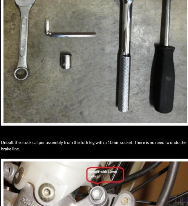
Unbolt the stock caliper assembly from the fork leg with a 10mm socket. There is no need to undo the brake line.
