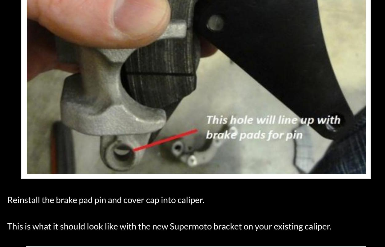
For optimum performance, we suggest you replace your brake pads at this time as well. New pads will help you achieve the performance gain you are looking for with the oversize rotor. Old pads that are worn to fit the existing rotor shape will not conform to the flatness of the new rotor and can hinder braking power.
