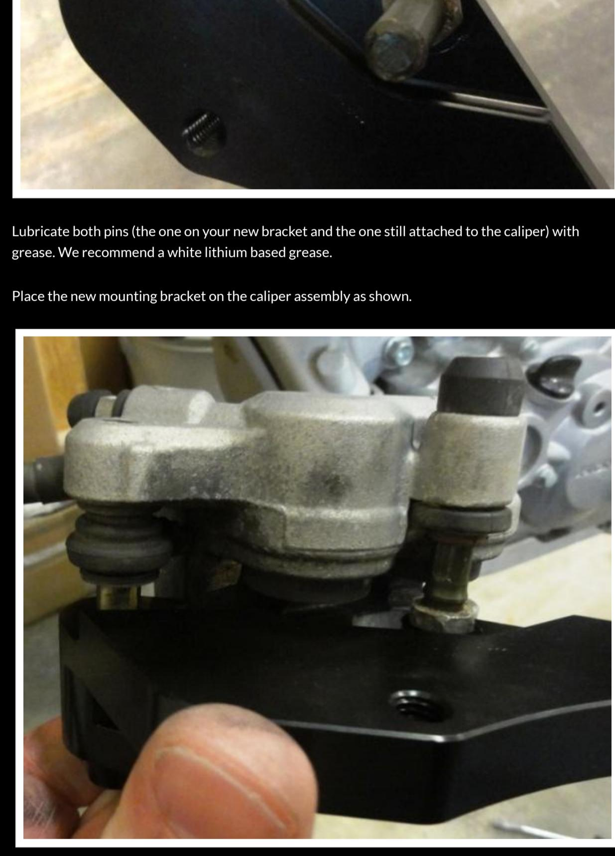
Next you will have to remove the mounting bracket portion because this is what we are going to replace. See the image below to help understand what piece you will be removing. With the pads removed it will slid apart on 2 floating pins.
