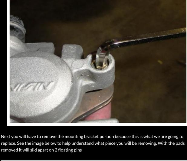
Next you will have to remove the mounting bracket portion because this is what we are going to replace. See the image below to help understand what piece you will be removing. With the pads removed it will slid apart on 2 floating pins
