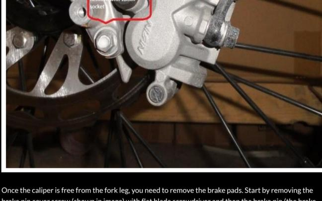
Once the caliper is free from the fork leg, you need to remove the brake pads. Start by removing the brake pin cover screw (shown in image) with flat blade screwdriver and then the brake pin (the brake pin holds the pads in the caliper). Once you remove the cover screw, you will see a 6mm Allen head bolt, remove that. The brake pads should now be easy to remove.
