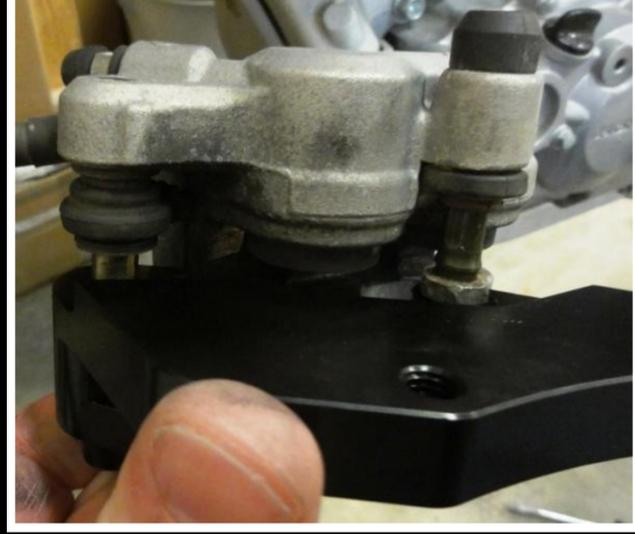
Reinstall the brake pad pin and cover cap into caliper.
