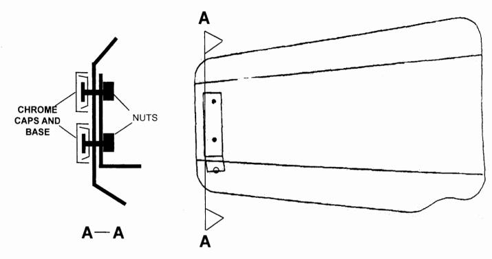
Assemble with hardware shown, with angle on bracket towards the curved knotch on hand warmer, curved knotch is designed to clear top Wind Wing if you have dual wings. If it still touches top wing, your handlebars may have been set too low. To raise the handlebars, remove the key cover and cover on center of handlebars, loosen the four bolts and raise bars till they clear. Tighten bolts and replace covers.
