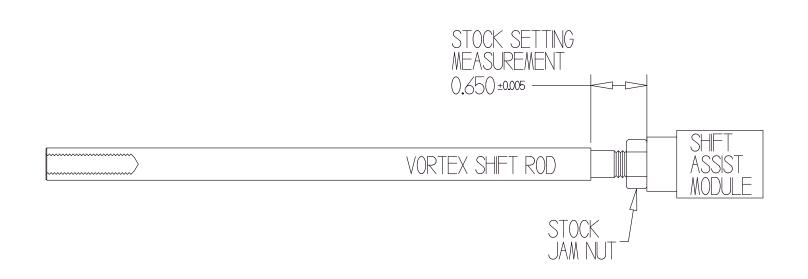
To ensure the correct operation of the shift assist system please install the Vortex Shift Rod (RS188C1 Or RS188C2) as shown in the diagram. Take great care to ensure that you have the system adjusted as shown to start. Once this is set please use the heim joints on both ends of the shift rod / shift assist assembly to adjust the length for pedal position.
