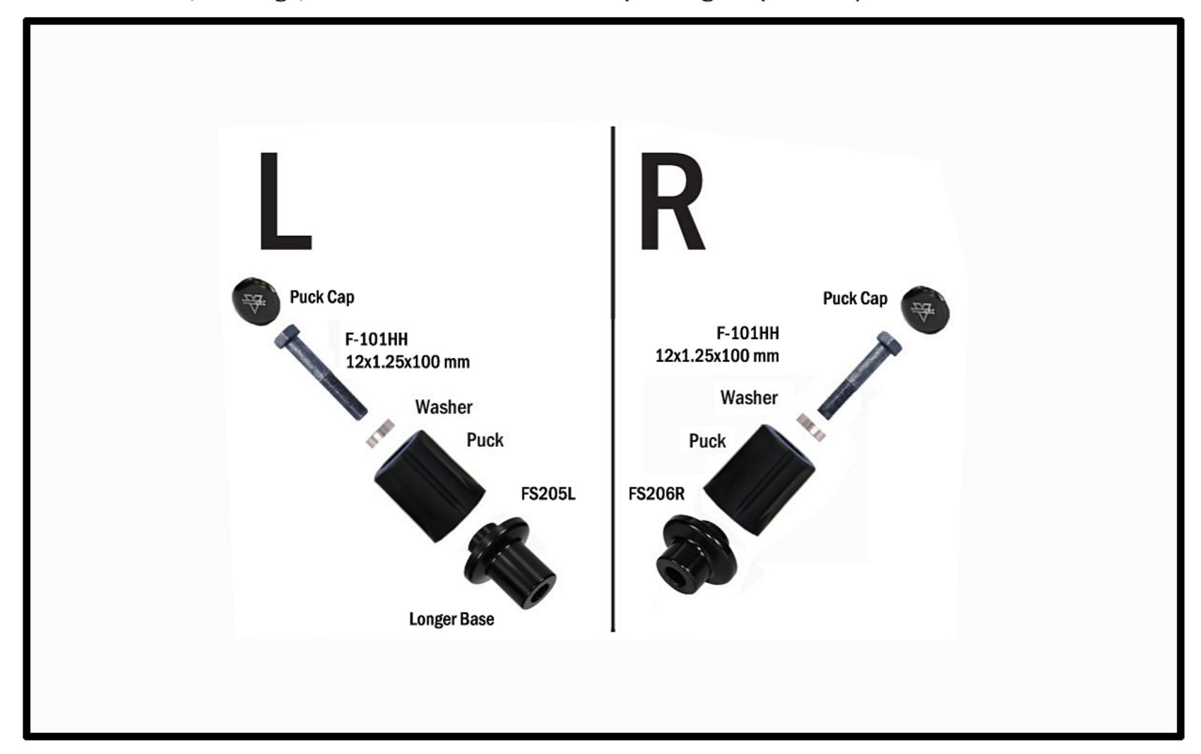
IMPORTANT: Washers will fit VERY snugly into Puck. Be sure that Washers are installed level as an unlevel installation can cause damage to the Puck. Use anti-seize grease on all bolts. Check bolts periodically for tightness. To be installed by a certified mechanic only. For race use only.
