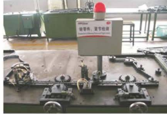
Inspection of missing parts
