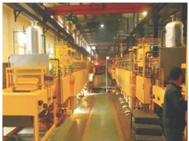
Automatic mesh belt conveyor furnace (Factory one)
