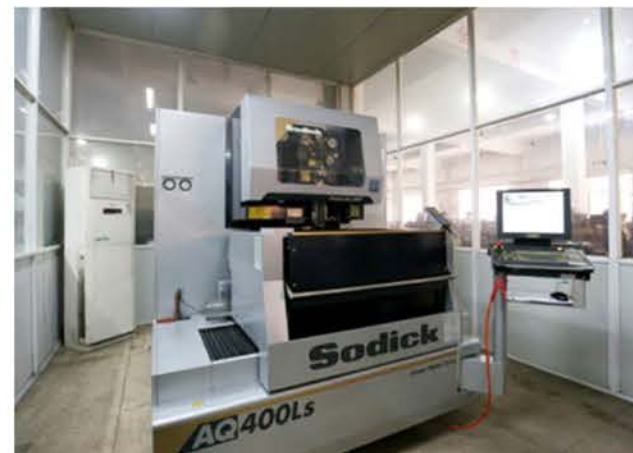
Japan-imported slow-feeding wire-cutting machine
