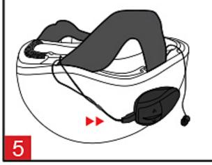
Connect speaker plug to the control unit, pushing plug in until the three ribs are no longer visible.
