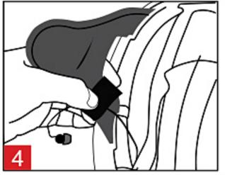
Position the earbud cable with the 3" Velcro strip. Note: Trim Velcro strip if necessary.
