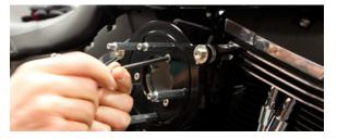
9. Install TBR air filter and face plate. Tighten the five socket head cap screws. Apply anti-seize to threads.
