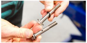
Install one o-ring onto each end of the oil-channel spacer.
