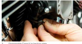
Disassemble Comp-V to backing plate.
