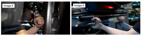
Remove allen screws holding OEM heat shield to OEM mufflers and separate muffler from heat shield. (Reference image 7) 8.
