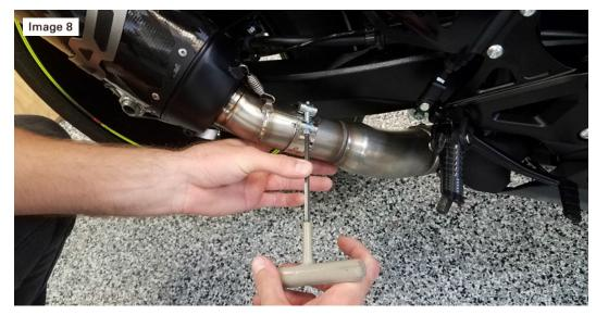
9. Before you run the bike, clean off all fingerprints and dirt, as any oily residue will etch the metal and become somewhat permanent when the system gets hot. Run the bike and enjoy. Check for gaps or leaks. After 50 to 100 miles, recheck all fasteners for tightness.
