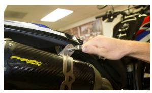
Before you run the bike, clean off all fingerprints and dirt, as any oily residue will etch the metal and become somewhat permanent when the system gets hot. Run the bike and enjoy. It is normal for some white smoke to appear the first time you start the bike. This is packing/manufacturing oil from inside the pipe burning off. Check for gaps or leaks. If you find a leak, a little high temperature silicon sealant should fix it. After 50 to 100 miles, recheck all fasteners for tightness.
