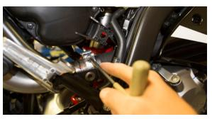
6. Using the included 8 x 75mm bolt, spacer, and 8mm nut – install the muffler with muffler clamp to the TBR slip tube. NOTE: Be sure to put the spacer in place on the bike before sliding the bolt through.
