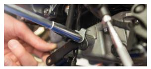
8. Loosely install the TBR slip tube and barrel clamp to the TBR headers.
