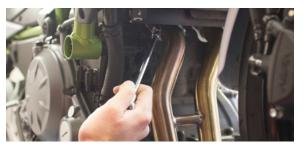
Remove O2 sensor routing bracket. Re-install side covers and check for clearance. When muffler is positioned tighten barrel clamp at header joint.
