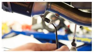
13. Reinstall O2 sensor onto TBR slip tube using supplied 12mm adapter kit and copper washer.
