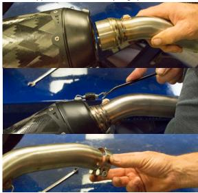
Install TBR muffler assembly to motorcycle using the supplied barrel clamp at header joint and OEM hardware.
