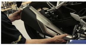
Remove header mounting hardware and remove header assembly.(the OEM bolts will not be re-used)
