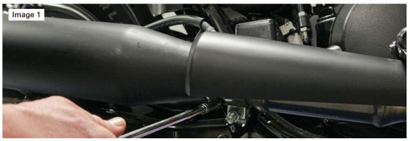
3. Remove two rear mount bolts. These will not be used with the TBR mufflers. (Reference image 2)
