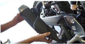
Attach TBR muffler to TBR slip tube using springs provided.
