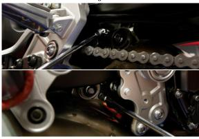
6. Remove OEM exhaust assembly.
