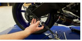
7. Re-route the O2 Sensor around the frame and along the engine.
