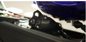
5. Remove the servo cap and disconnect the cables.
