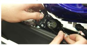
6. Remove the cables and put the servo back.
