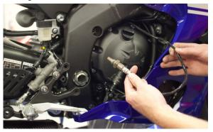
8. Before you run the bike, clean off all fingerprints and dirt, as any oily residue will etch the metal and become somewhat permanent when the system gets hot. Run the bike and enjoy. It is normal for some white smoke to appear the first time you start the bike. This is packing/manufacturing oil from inside the pipe burning off. Check for gaps or leaks. If you find a leak, a little high temperature silicon sealant should fix it. After 50 to 100 miles, recheck all fasteners for tightness.
