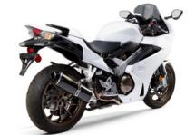
**INTERCEPTOR/VFR800** Slip-On Exhaust System - Designed NOT to be used with saddle bags.
