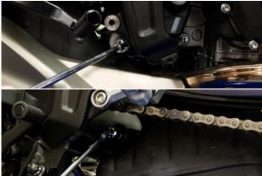
5. Remove O2 sensor from OEM muffler.
