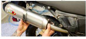
Install S1R mounting hardware bolt, washer, clamp, spacer, and nut. Securely tighten.
