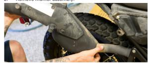
Attach S1R muffler to TBR slip tube using supplied hook springs. Loosely install barrel clamp onto slip tube inlet.
