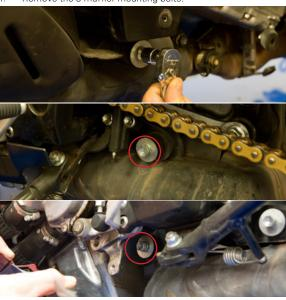
5. Remove OEM muffler assembly
