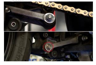
Remove lower rear set bracket bolt and install new 8x40mm socket head cap screw provided.
