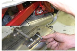
Remove the rubber grommet and inserts from the frame where the stock muffler mounted on the left side.
