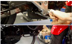
9. Install TBR header assembly using OEM hardware and gasket.
