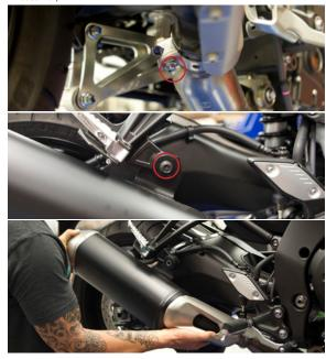
3. Remove OEM muffler mount bracket from right passenger peg.
