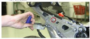
Remove right side driver's footpeg bolts and carefully remove the exhaust tube heat shield behind.
