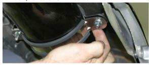
23. Securely tighten barrel clamp.
