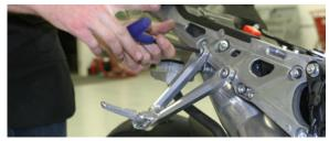
Replace tail light assembly, reconnect wiring and replace rear cowling, passenger & driver seats.
