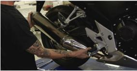
Install TBR slip tube and TBR supplied barrel clamp. Leave loose for now.
