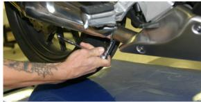
Remove OEM muffler mounting hardware. Save for use with TBR muffler.
