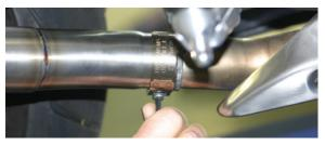
Before you run the bike, clean off all fingerprints and dirt, as any oily residue will etch the metal and become somewhat permanent when the system gets hot. Run the bike and enjoy. It is normal for some white smoke to appear the first time you start the bike. This is packing/manufacturing oil from inside the pipe burning off. Check for gaps or leaks. If you find a leak, a little high temperature silicon sealant should fix it. After 50 to 100 miles, recheck all fasteners for tightness.
