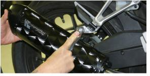
8. Check for clearance and alignment, then tighten all the bolts in this order: X-ring bolts, muffler mount, and finally barrel clamp.
