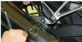
Remove OEM muffler assembly. OEM gasket will not be used with TBR exhaust.
