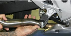
Attach muffler to TBR slip system using the supplied X-ring, 8x20mm socket head cap screws and lock washers that are provided, leave loose for now. Slide rubber lined muffler clamp and barrel clamp on and install to bike.
