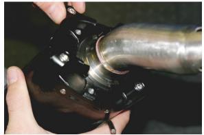
Attach TBR muffler bracket using OEM mounting hardware.
