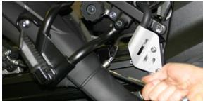
5. Loosen rear exhaust clamp. This is accessible from the left side of the bike.
