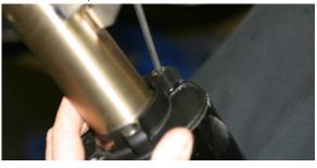
Loosely attach muffler to bike using the OEM hardware on slip-tube mount and install muffler clamp using the supplied bolt and spacer.
