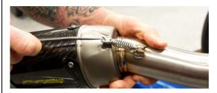
Reinstall right side rear set. Torque hardware to OEM 14. Slide TBR slip tube and muffler assembly onto header using supplied barrel clamp. Leave loose for now.
