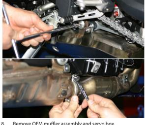
Remove OEM muffler assembly and servo box.
