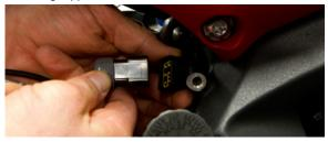
17. Attach servo eliminator to brake lines using supplied zip-tie.
