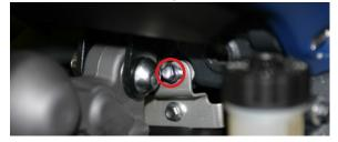
Temporarily remove right side rear set mounting hardware 6. to ease removal of servo box.
