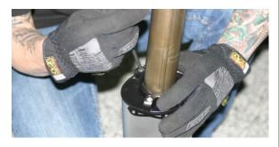
6. Install TBR muffler assembly.
