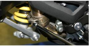
4. Remove stock muffler assembly.
