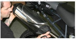
5. Attach TBR slip tube to TBR muffler using the 2 piece X-Ring and 6x14mm socket head cap screws with lock washer that are provided. Leave loose enough to make some adjustments on the motorcycle.
