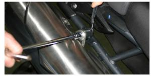
3. Loosen pipe joint clamp.
