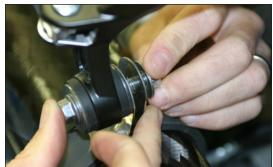
Check alignment of muffler and tighten the 4 6x20mm socket head cap screws. Then tighten barrel clamp and lastly tighten muffler mount.
