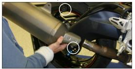
Install TBR muffler to slip-tube shown using the supplied 2-piece X-Ring and bolts with lock washers, keep loose for now.
