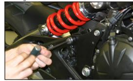
4. Remove muffler mounting hardware.
