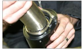
Slide the supplied rubber-lined muffler canister clamps over the TBR muffler canisters. Place the supplied barrel clamp around the end of the TBR slip-on tube, slide the slip-tube onto the stock collector.
