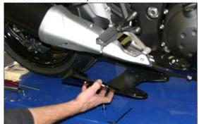
Remove left and right stock exhaust canisters, retain OEM hardware for TBR installation.
