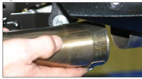
Attach the muffler canisters to the bike using the OEM hardware.
