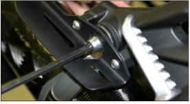
Check to be sure that both exhausts are positioned and aligned correctly. Once you are satisfied with the position of the exhaust, tighten the V.A.L.E. X-Ring, then the barrel clamp followed lastly by the muffler canister clamp.
