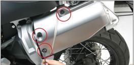
3. Remove OEM exhaust by removing mounting bolt and loosening mide tube bracket.
