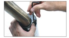
Install TBR muffler assembly to motorcycle with the rubber lined muffler clamp on muffler and barrel clamp on slip-tube. Muffler clamp attaches to outside of muffler bount bracket with supplied bolt, nut and washer.
