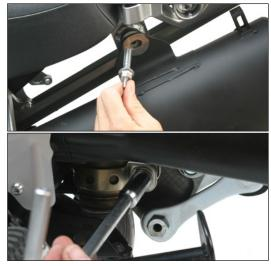
Install TBR muffler bracket with OEM mount bolt and nut, leave loose for now.
