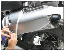
Before you run the bike, clean off all fingerprints and dirt, as any oily residue will etch the metal and become somewhat permanent when the system gets hot. Also, remove any protective plastic from the name badges on the muffler canister(s) or the muffler clamp(s). Run the bike and enjoy. It is normal for some white smoke to appear the first time you start the bike. This is packing/manufacturing oil from inside the pipe burning off. After 50 to 100 miles, recheck all fasteners for tightness.
