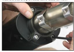
Slide barrel clamp over slip-tube and install muffler assembly to bike.
