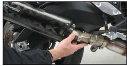
Slide rubber lined muffler clamp over muffler assembly and loosely attach to rear lower passenger foot mount using supplied 8x16mm bolt.
