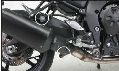
3. Remove OEM muffler mount bracket.
