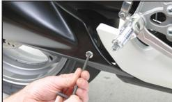
3. Remove OEM muffler assembly.
