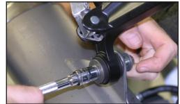
Remove header assembly including butterfly cables, loosen radiator bolts for better access.
