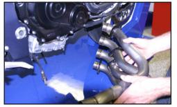
Attach muffler to TBR slip system using the supplied X-ring, 6x20mm socket head cap screws and lock washers that are provided, leave loose for now. Slide rubber lined muffler clamp and barrel clamp on and install to bike.
