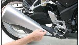
3. Install supplied muffler mount to right side rear footpeg using supplied 6x45mm bolt and nut.
