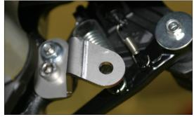
8. Attach TBR muffler to slip-on tube using the 4 6x20mm S.H.C.S. and lock washers provided. Leave loose for now.
