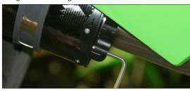
13. Tighten muffler mounting clamp, then barrel clamp.
