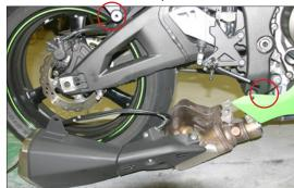
Attach TBR muffler to slip-on tube using the 4 6x20mm S.H.C.S. and lock washers provided. Leave loose for now.
