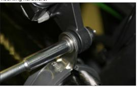
Check alignment and tighten muffler and the 4 6x20mm V.A.L.E.™ S.H.C.S.
