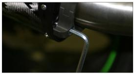
10. Tighten barrel clamp.
