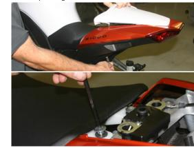
3. Remove support bracket under main seat assembly.
