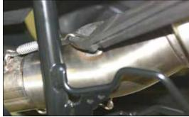
3. Remove muffler mounting bolt and decorative washer, set aside to re-use washer later.
