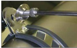
6. Align muffler and tighten the 4 X-Ring bolts.
