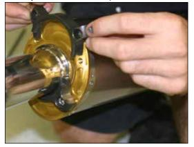
Attach muffler assembly to motorcycle using the OEM springs and suplified muffler clamp. Use the supplied 8x20mm socket head cap screw and OEM washer to secure muffler clamp.
