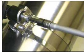
Attach TBR slip tube to TBR muffler using the 2 piece X-Rings and 6x14mm socket head cap screws with lock washer that are provided. Leave loose enough to make some adjustments on the motorcycle.
