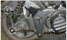
Install TBR muffler to TBR header pipe using the 6x14mm socket head cap screws and lock washers provided, leave loose for now.
